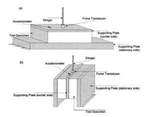
Fig. 1. Test arrangement for experiment in (a) tension compression and (b) shear.
