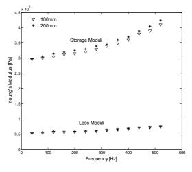
Fig. 7. Young's modulus for samples with lubricated boundaries on sides.
