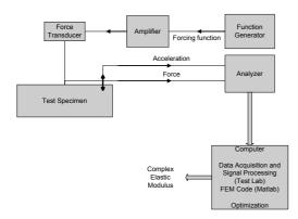
Fig. 2. Schematic of Experimental/numerical procedure to determine the complex elastic moduli.
