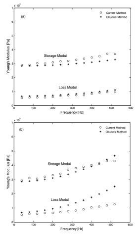
Fig. 6. Measurements with sample in tension compression (a) Transfer function, (b) Young's modulus.
