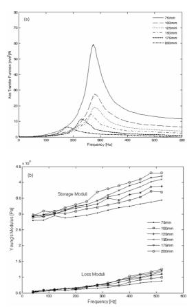
Fig. 5. Measurements with sample in tension compression (a) Transfer function, (b) Young's modulus.
