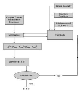
Fig. 3. Block diagram of the experimental/numerical procedure for determining the material properties.
